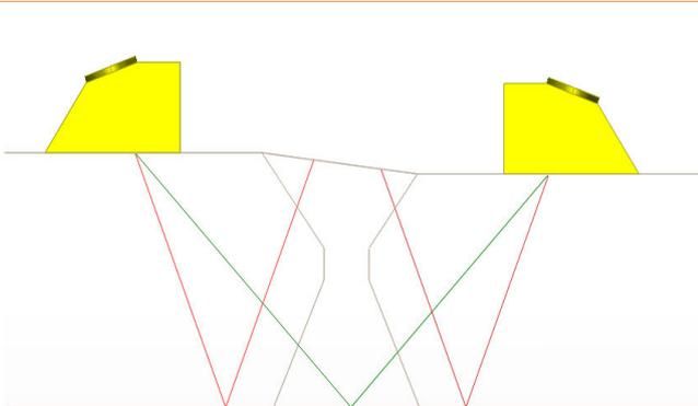
Figure 1: An example of one of the models created in the Civa NDE software.
